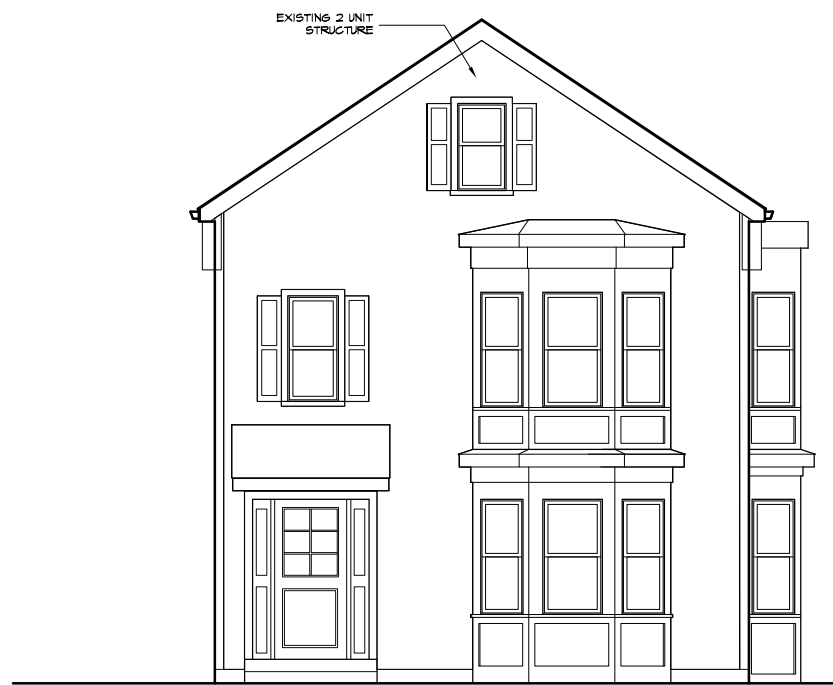
○ EXISTING SOUTH ELEVATION 1/4" = 1'-0"
